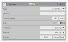
Click Bind under the **[RF System]** menu and select the required Channel/Telemetry working mode, then the radio will enter the Bind mode.
